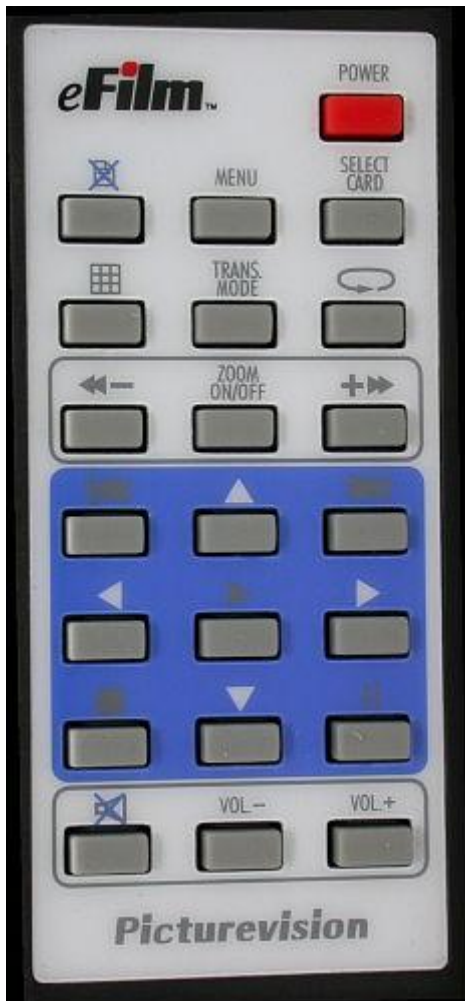
Here's the Picturevision's infrared remote control, across the top are the Power, Delete, Menu, Card Select, Thumbnail, Transition, Repeat, Zoom Out, Zoom on/off and Zoom In buttons.
